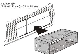
2 When the mounting sleeve is in the correct position, bend several mounting *claws* outward to achieve a tight fit and lock the mounting sleeve into place.
